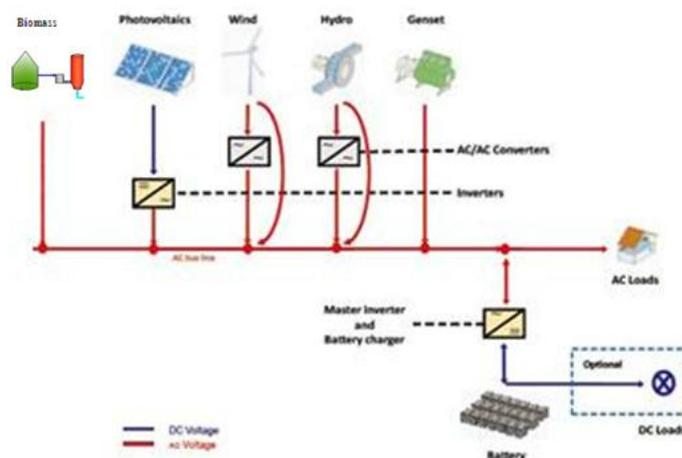
Fig.2. AC bus bar coupled Hybrid mini-grid [6]
