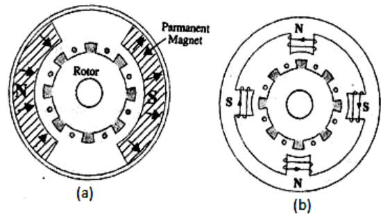
Fig.5. Construction of permanent magnet in PMDC.
