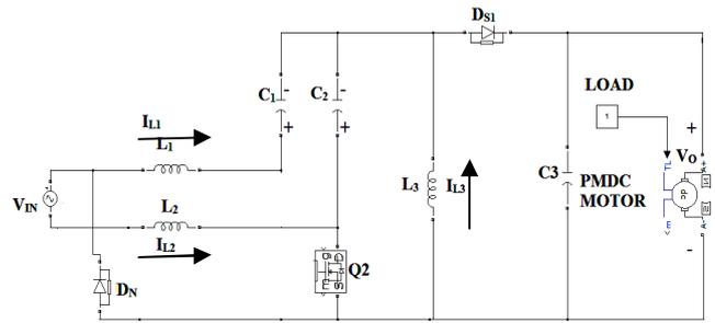
Fig.9. During negative half cycle, switch Q2 turn on and Q1 turn off condition.
