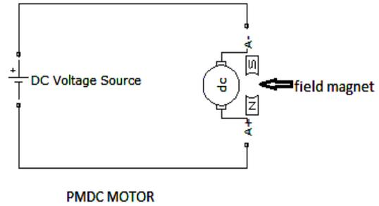
Fig.4. Permanent magnet DC motor
