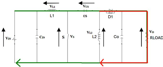
Fig.3: Current flows during switch is turn off condition.
