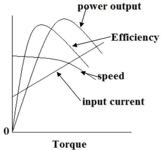
Fig.6. Charteristics of PMDC motor.
