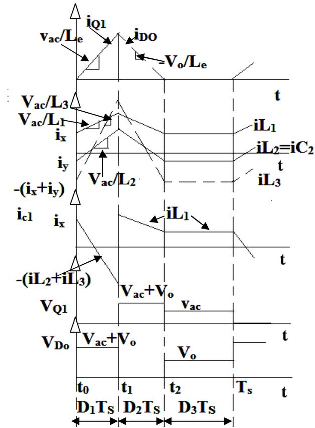
Fig.11. Theoretical waveforms in DCM of proposed converter
