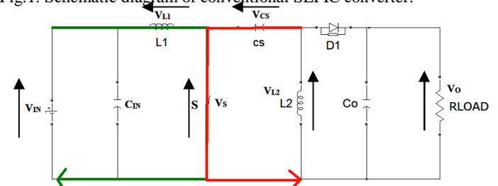
Fig.2: Current flows during switch is turn on condition
