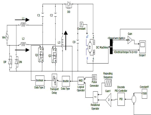
Fig.7. Bridgeless SEPIC converter circuit diagram.
