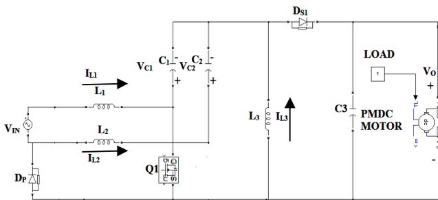
Fig.8. During positive half cycle, switch Q1 turn on and Q2 turn off condition.
