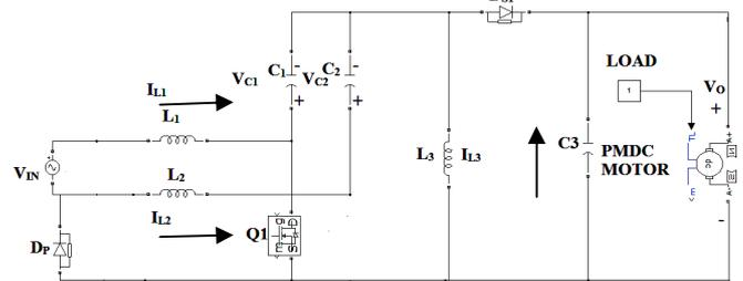
Fig.10(a). During positive half cycle, switch Q1 turn on and Q2 turn off condition.
