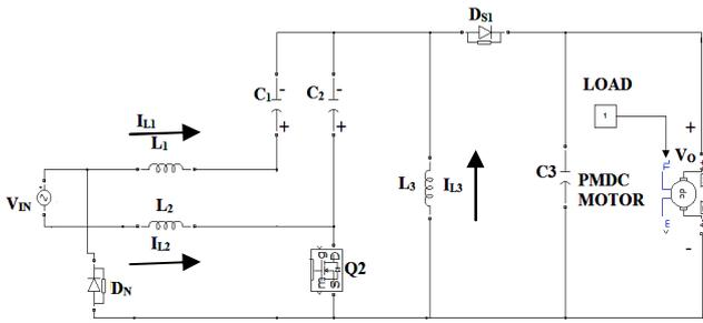
Fig.10(b).During positive half cycle, switch Q1 turn on and Q2 turn off condition
