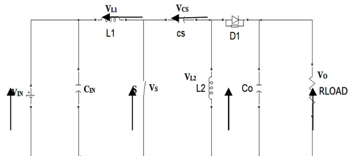
Fig.1. Schematic diagram of conventional SEPIC converter.
