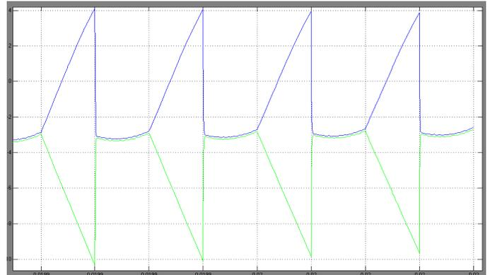
Fig.13.Capacitors C<sub>1</sub> and C<sub>2</sub> voltage waveforms.
