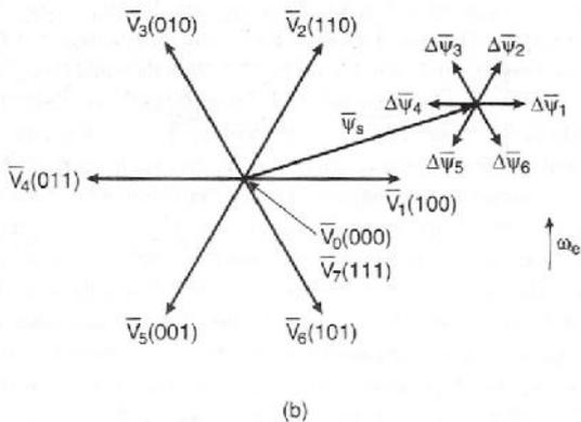
Fig 6: In principle the DTC method selects one of the six nonzero and two zero voltage
