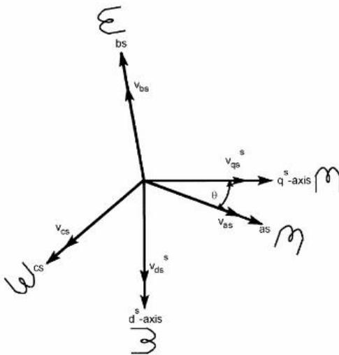
Fig 2. Stationary frame a~b~c to d<sup>s</sup>~q<sup>s</sup> axes transformation.
