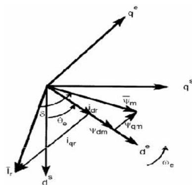
Fig.3: (a) Stationary frame d<sup>s</sup> - q<sup>s</sup> to rotating frame de - q<sup>e</sup> ; (b) Flux and current vectors d<sup>e</sup> - q<sup>e</sup>.
