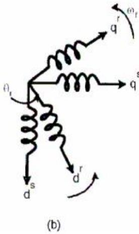
Fig 1: (a) Coupling effect in three-phase stator and rotor windings of motor; (b) Equivalent two-phase machine.
