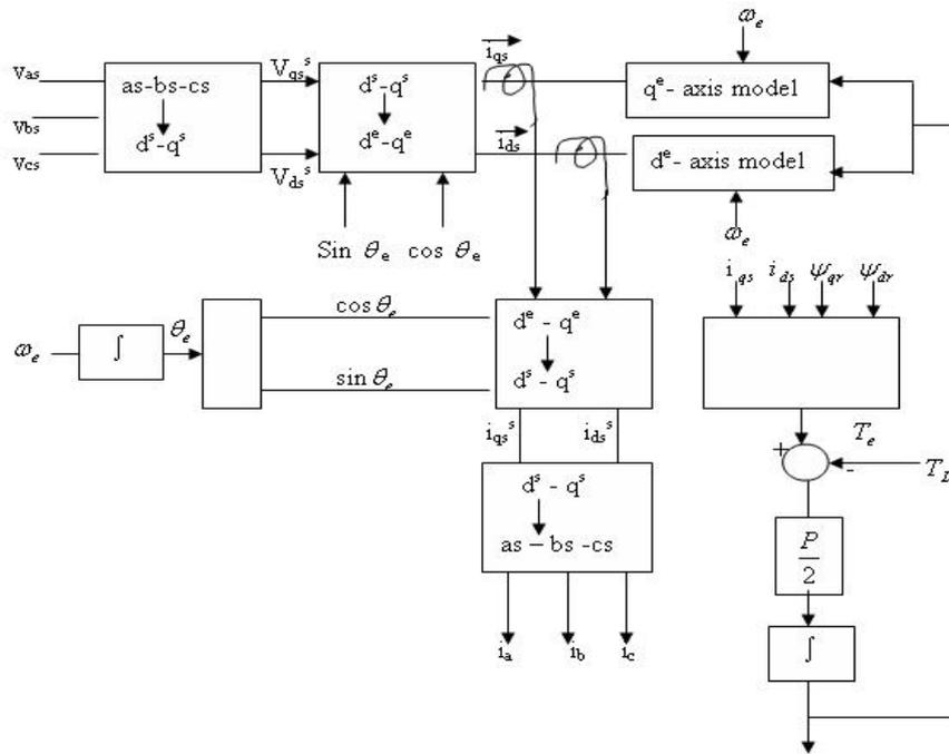
Fig 4. Synchronously rotating frame machine models with input voltage and output current transformations.
