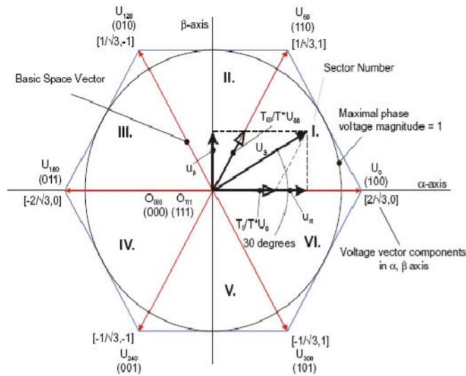
Fig. 5: SVM and different possible switching voltage vectors
