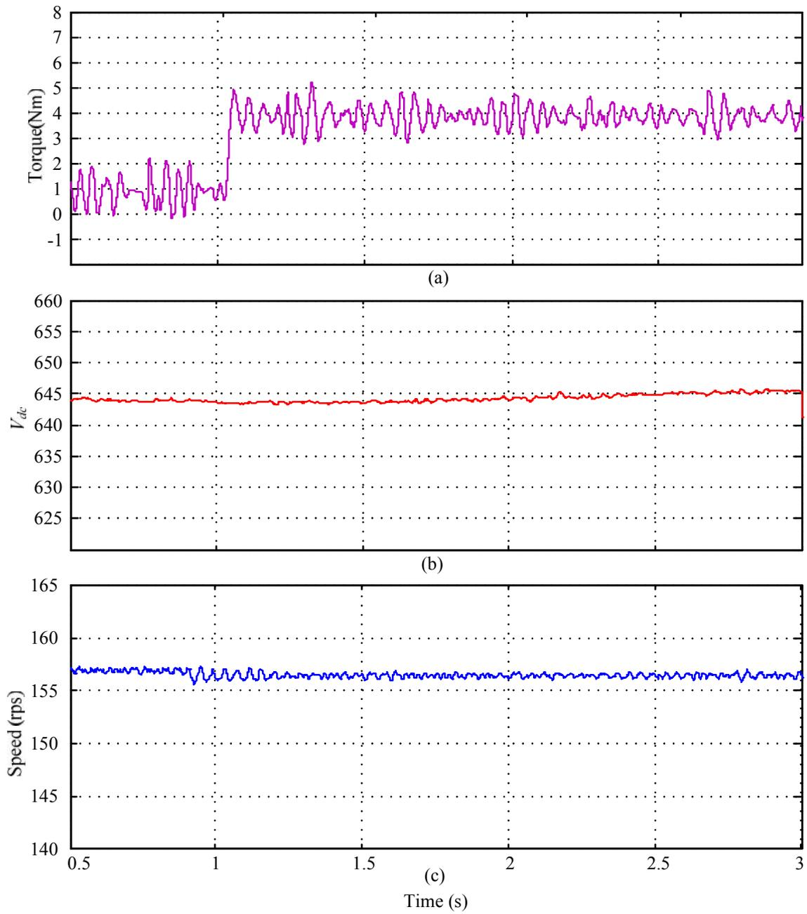
Fig. 10: (a) Electromagnetic torque, (b) dc-link voltage, (c) Speed of induction motor.
