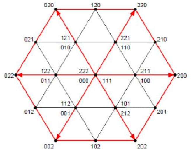
Fig 8: Inverter voltage vectors and corresponding stator flux variation in time  $\Delta t$ .
