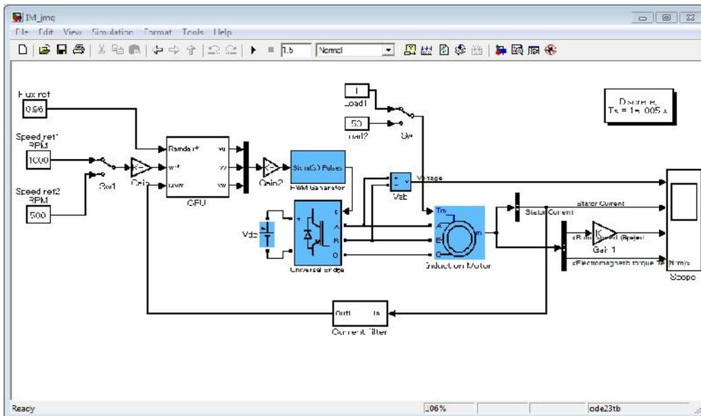
Fig. 9: Matlab block diagram of proposed model.
