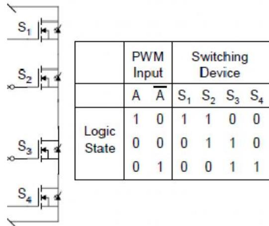
Fig. 7: 1-leg of 3-level inverter and corresponding switching pattern.
