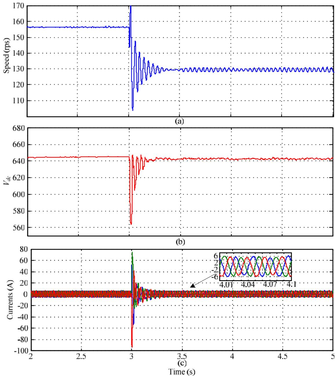
Fig. 11: (a) Speed of induction motor, (b) dc link voltage, (c) stator currents.
