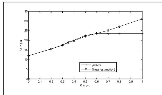
Figure. 3: Reactive power generation at bus 6 as a function of the per unit reduction in power flow.
