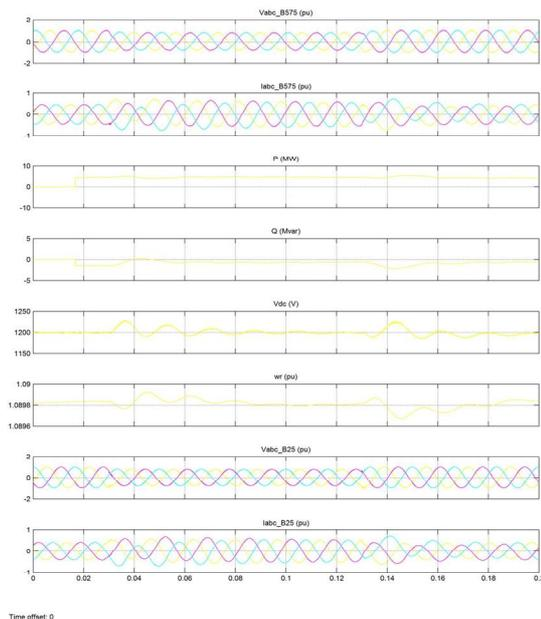
Fig 11: Waveforms for wind speed 13m/s
