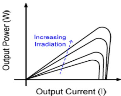
Fig 6. PV cell power characteristics
