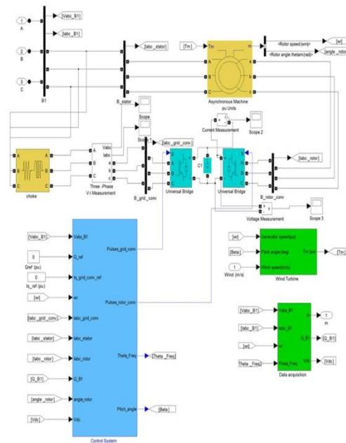
Fig 9: Matlab model of WECS
