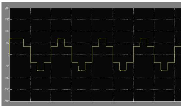
**Fig 2: Current waveform of 3 level inverter**
