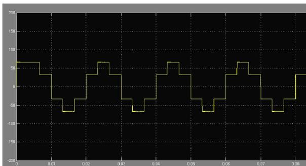
**Fig 3: Voltage waveform of 3 level inverter**
