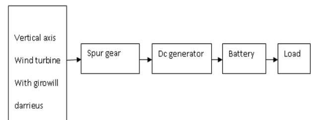
Figure.1-Wind power generation system.
