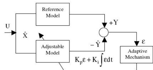
Fig. 1. Basic configuration of a parallel model reference adaptive system.
