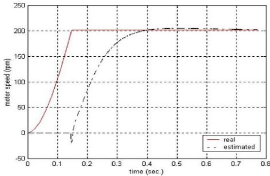
Fig. 5. Behaviour of speed estimation at  $K_{p3} = 5$ ,  $K_{i3} = 250$ .
