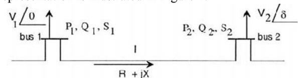
Fig. 1. Two-bus power system model
