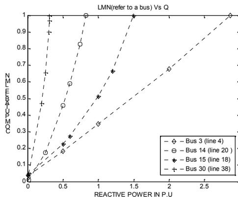
Fig. 7. LMN Vs Reactive load variation (Q)
