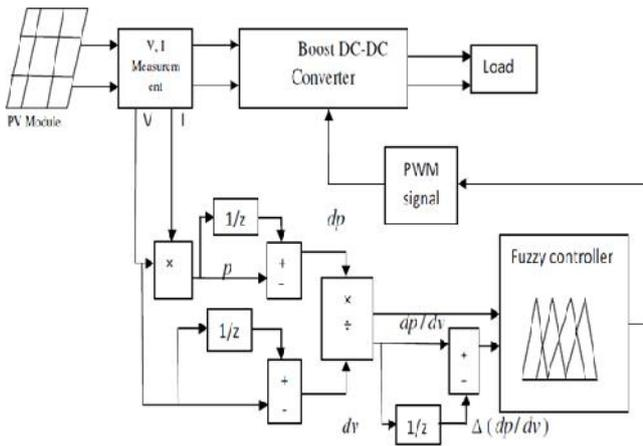
Fig.6 Block diagram of FLC based MPPT control
