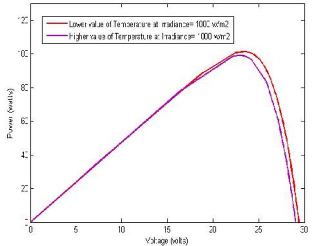
Fig.12 P-V characteristics of PV array with different temperature and at constant irradiance
