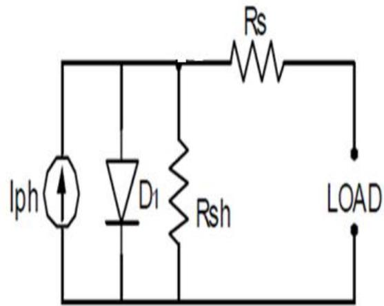
Fig.1 PV Cell Circuit Model
