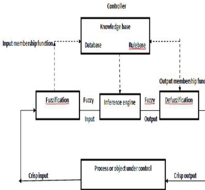
Fig.7 Internal structure of Fuzzy Logic Controller
