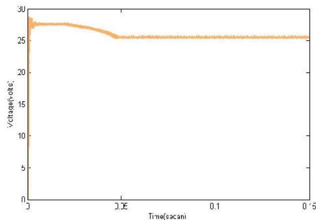
**Fig.14 (b)** PV array output Voltage for FLC MPPT control
