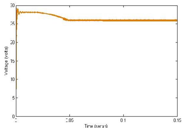
**Fig.13(b)** PV array output voltage for P&O MPPT technique
