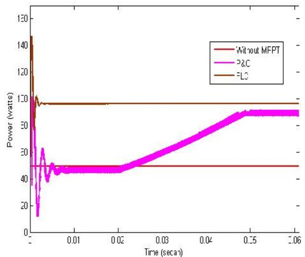
**Fig.15** PV array output power waveform with and without MPPT
