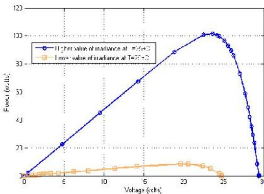
Fig.10 P-V characteristics of PV array with different irradiance and at constant temperature
