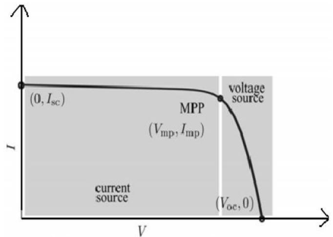
Fig.2 Maximum Power Point ( $V_{mp}, I_{mp}$ ).
