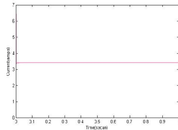
**Fig.14 (a)** PV array output current for FLC MPPT control
