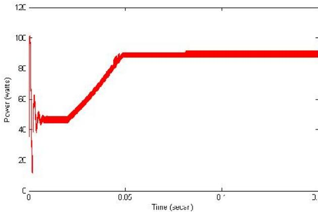
**Fig.13(c)** PV array output power for P&O MPPT technique
