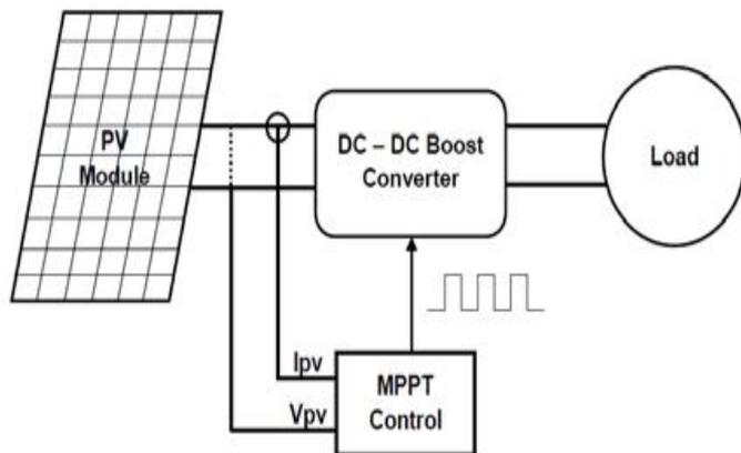
Fig.4 Block diagram of P&O MPPT technique
