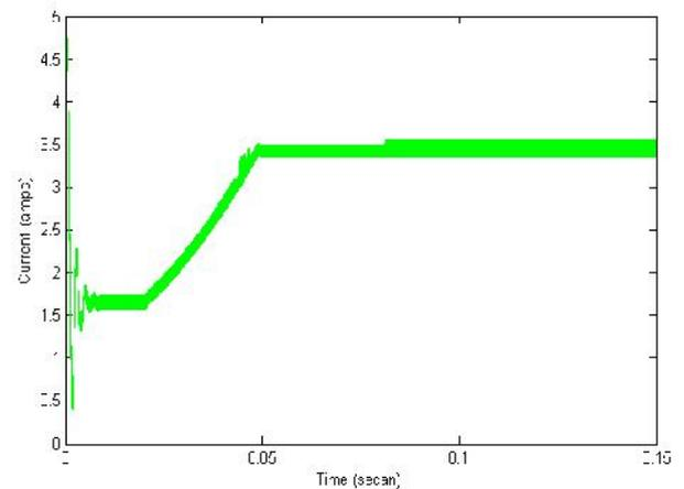
Fig.13(a) PV array output current for P&O MPPT technique
