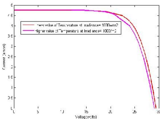
Fig.11 I-V characteristics of PV array with different temperature and at constant irradiance
