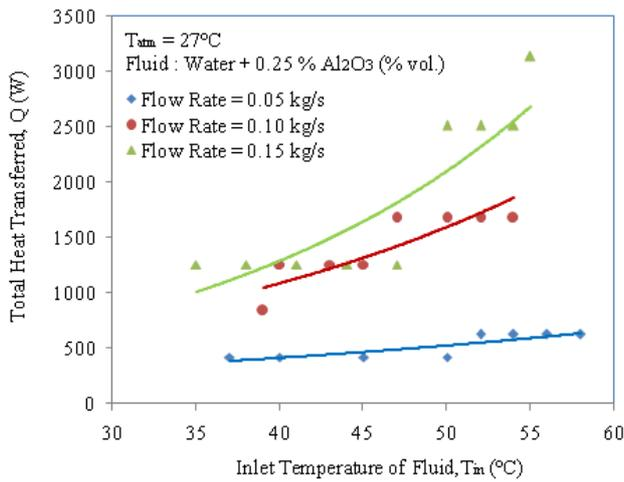
Fig 3. The influence of inlet temperature and flow rate of Al<sub>2</sub>O<sub>3</sub> nanofluid (0.25 % Vol) on the total heat transferred from radiator
