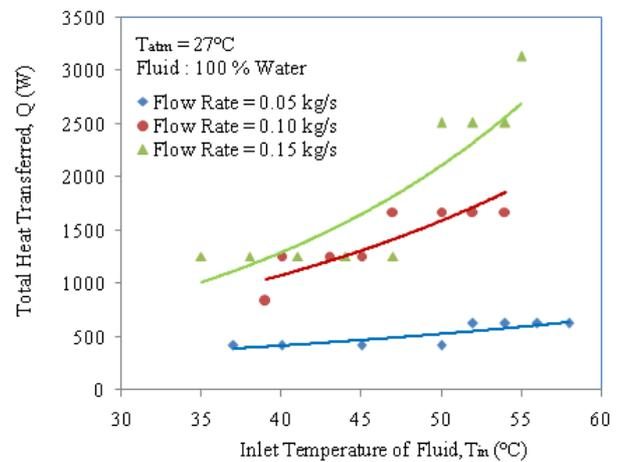
Fig 2. The influence of inlet temperature and flow rate of water coolant on the total heat transferred from radiator
