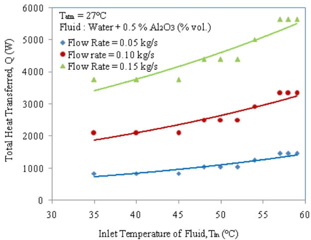
Fig 4. The influence of inlet temperature and flow rate of Al<sub>2</sub>O<sub>3</sub> nanofluid (0.50 % vol) on the total heat transferred from radiator
