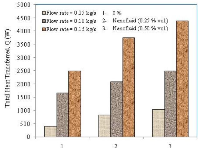
Fig 5. Effect of flow rate and concentration of nanofluid on the total heat transferred
