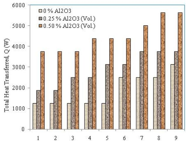
Fig 6. Effect of nanofluid concentration of nanofluid on the total heat transferred for varying inlet temperature
