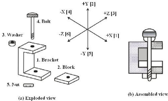
Figure 2. An example of assembly of a mechanical connector in Cartesian coordinate system
