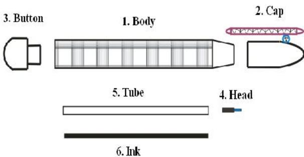
Figure 3. Exploded view of a ball-point pen assembly
