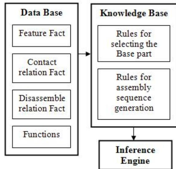
Figure 1. Overall structure of the expert system module based on assembly sequence planning
