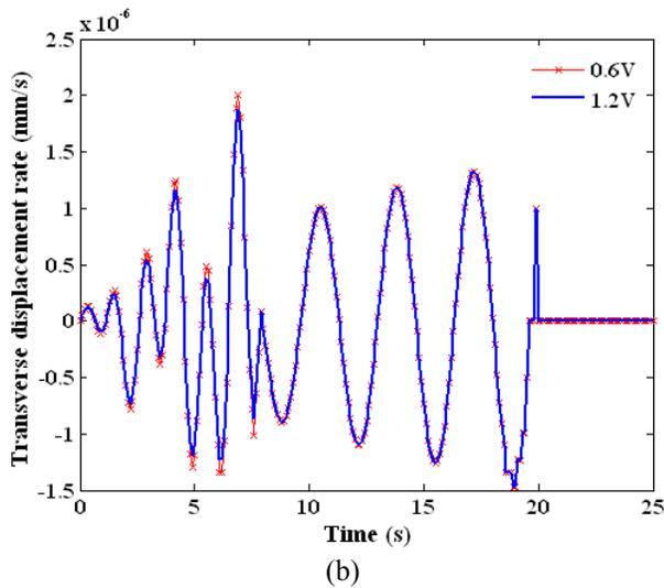
Figure 7. Tip velocity of the actuator combining first two modes i.e. response without delay  $T=0s$
