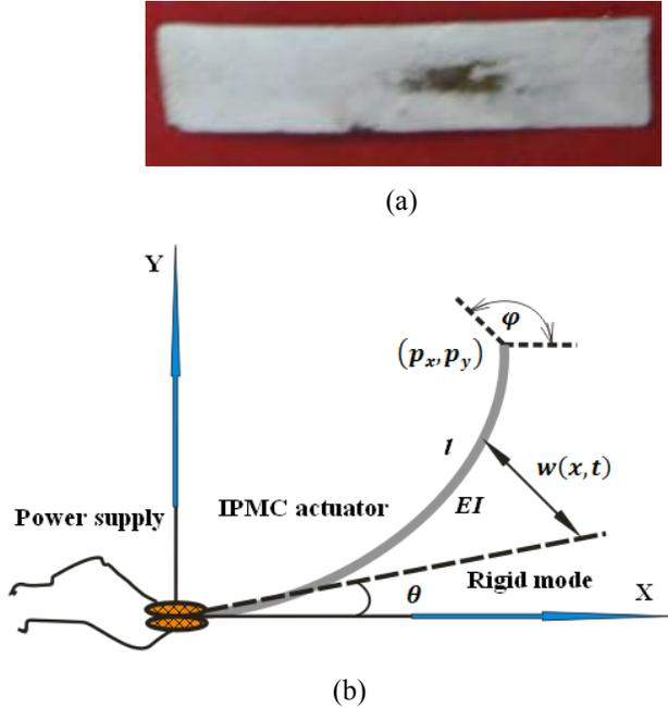
Figure 1. (a) Fabricated Ag-IPMC actuator (b) Schematic of IPMC actuator under an input voltage V
