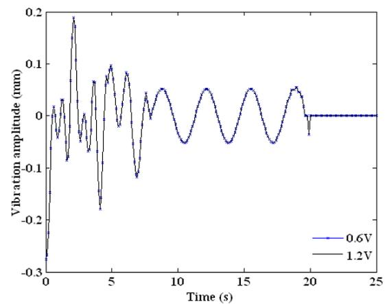
Figure 5. Delay free ( $T=0s$ ) vibration response of the actuator combining primary three modes (ODEs)
