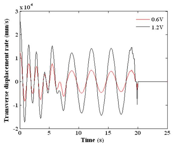
Figure 6. Rate of change of transverse displacement of the actuator combining primary two modes with a delay  $T=1s$
