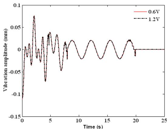
Figure 8. Vibration response of the actuator combining primary 3 modes with delay  $T=0.5s$  (DDEs)
