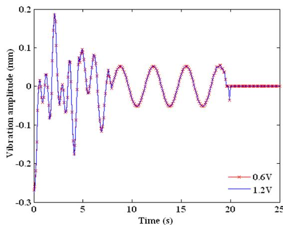
Figure 4. Vibration response of the actuator combining primary three modes with a delay of  $T=1s$  (DDEs)
