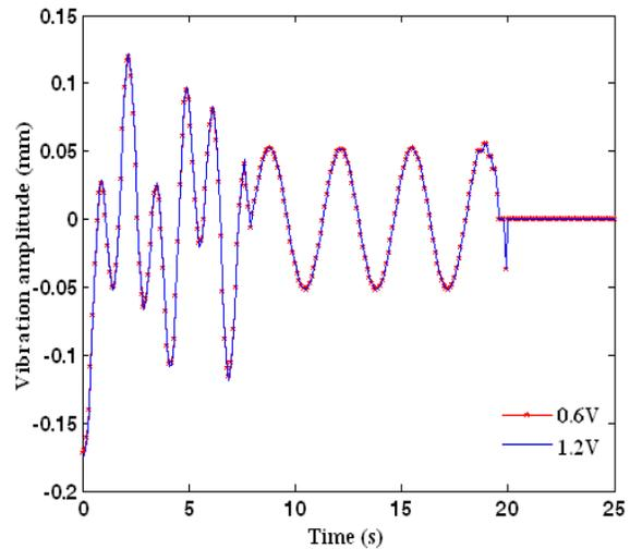
Figure 2. Vibration response of the actuator combining primary two modes with a delay  $T=1s$  (DDEs)
