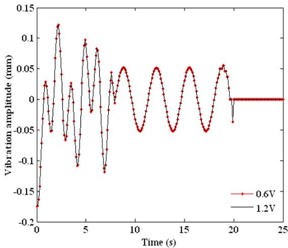
Figure 3. Vibration response of the actuator combining primary two modes without delay (ODEs) i.e.  $T = 0s$
