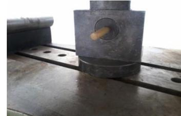
**Fig XVII: Specimen Held for Shear Test**
