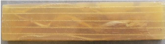
**Fig X: Bending Specimen**
