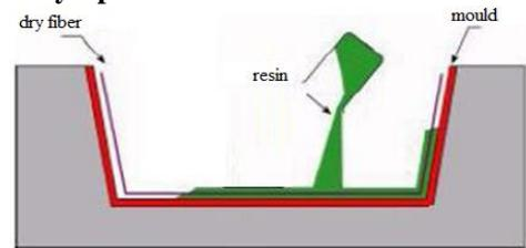
**Fig VIII: Hand Lay-Up Process**
