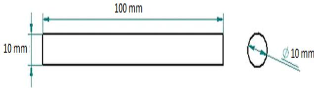
**Fig V: Shear Test Mould Made of Wood with Dimensions**
