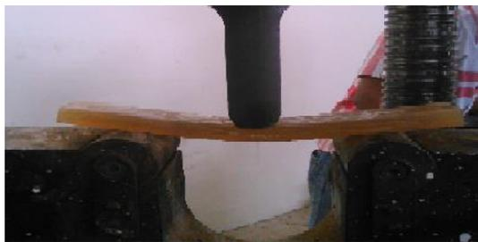
**Fig XIX: Specimen Held for Bending Test**
