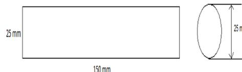
Fig II: Tensile Test Mould Made of Wood with Dimensions
