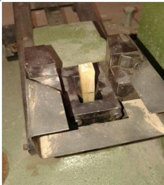
**Fig XVI: Specimen Held for Impact Test**
