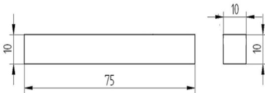
**Fig VI: Impact Test Mould Made of Wood with Dimensions**
