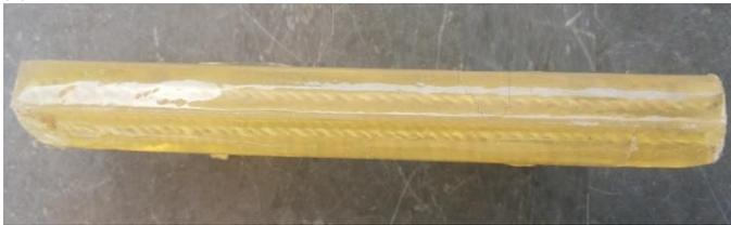
**Fig XI: Shear Specimen**
