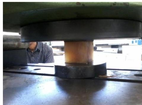
**Fig XVIII: Specimen Held for Compression Test**
