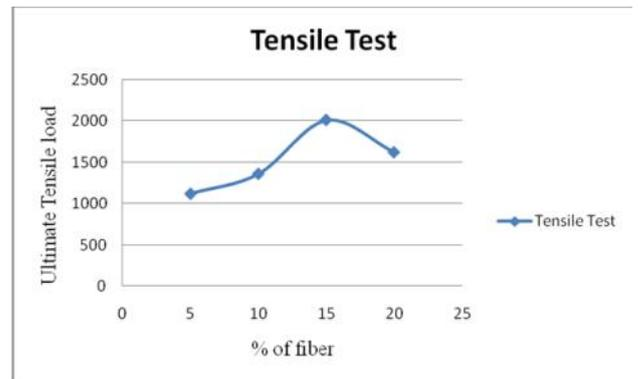
Fig. No 5.1 percentage of fiber Vs Ultimate load
