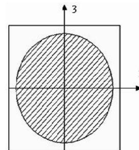
**Fig.4.2:** isolated Unit Cells of Square packed array
