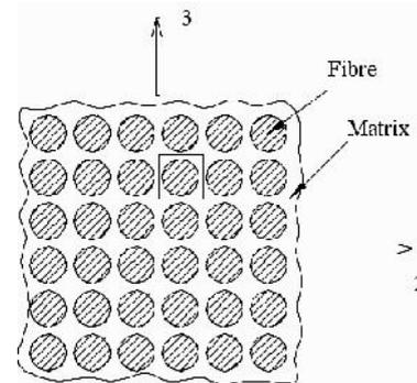
**Fig.4.1:** Concept of Unit Cells
