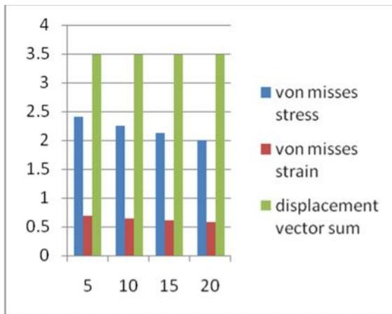
Fig 5.16 volume fraction of fiber Vs von misses stress, strain, displacement vector sum
