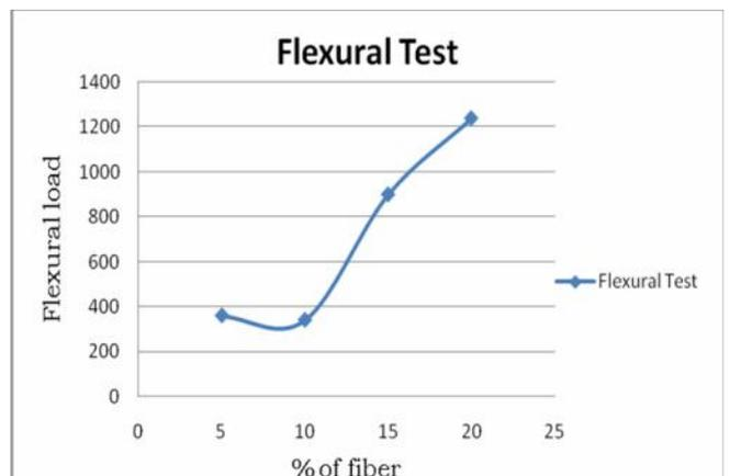
figure 5.2 Percentage of fiber Vs Flexural load
