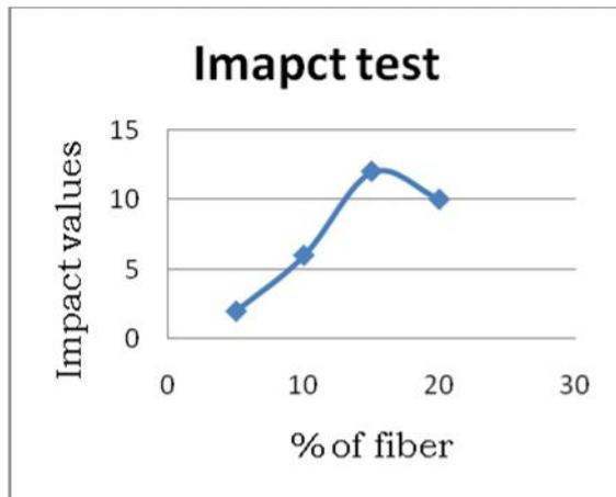
Fig . No 5.3 % of fiber Vs Impact values
