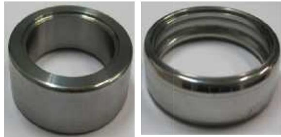
Figure 2 Final ring workpiece (right) rolled from the blank ring (left)
