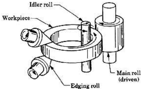
Figure 5 Schematic of a radial-axial ring rolling mill
