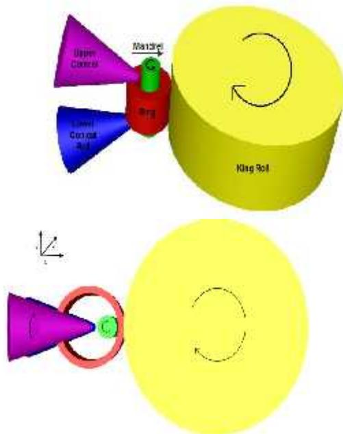
Figure: 1. (a) 3-D View of Ring Rolling Process, (b) Schematic View of Ring Rolling Process
