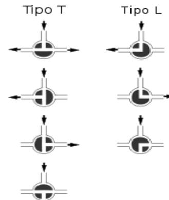
Fig. 1 WAY BALL VALVE L-SHAPED BALL RIGHT, T-SHAPED LEFT
