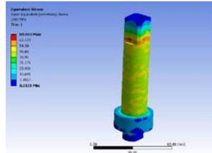
Fig.12 stress induced in the stem
