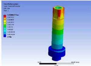
Fig.11 Deformation in stem
