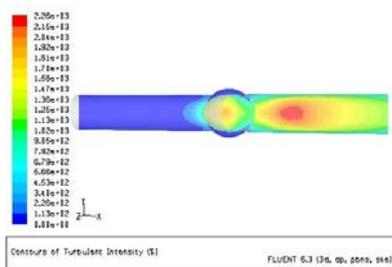
Fig.17 Turbulent intensity
