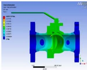
Fig.9 Deformation of the body
