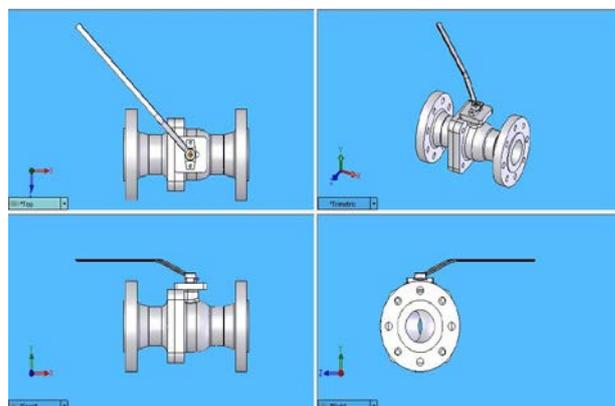
Fig.5 Top view, Front view, Right side view & Trimetric view of 4" 600# Ball Valve
