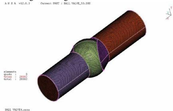
Fig.7 Domain meshing by using TGRID
