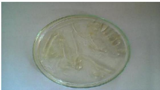
**Figure (5) Solution is cast on polythiophene doping PVA thin film**
