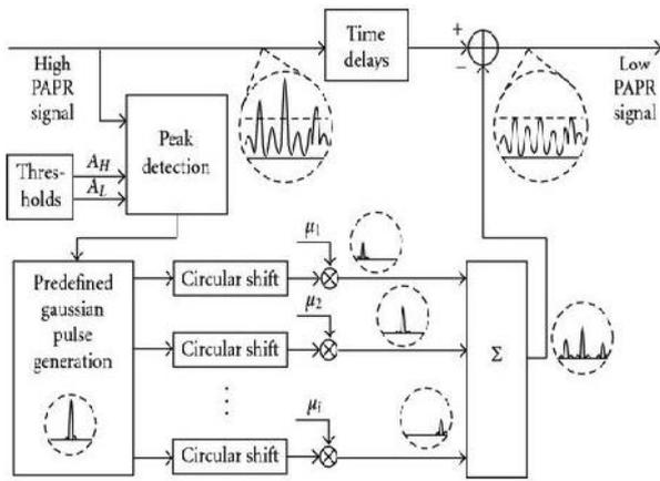
Fig.2. Gaussian pulse based Tone Reservation for Reducing PAPR of OFDM signal.
