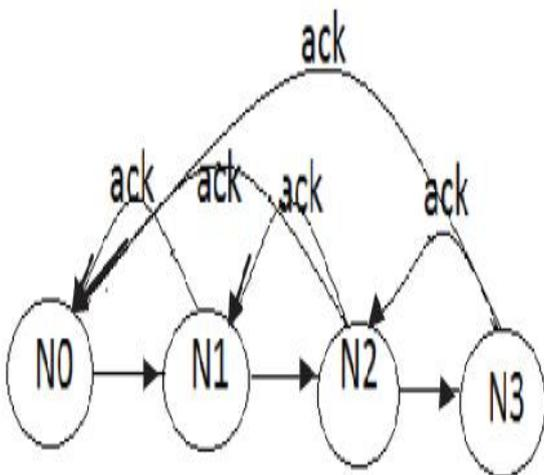
Fig.3.3 Node transmission and acknowledgement passing
