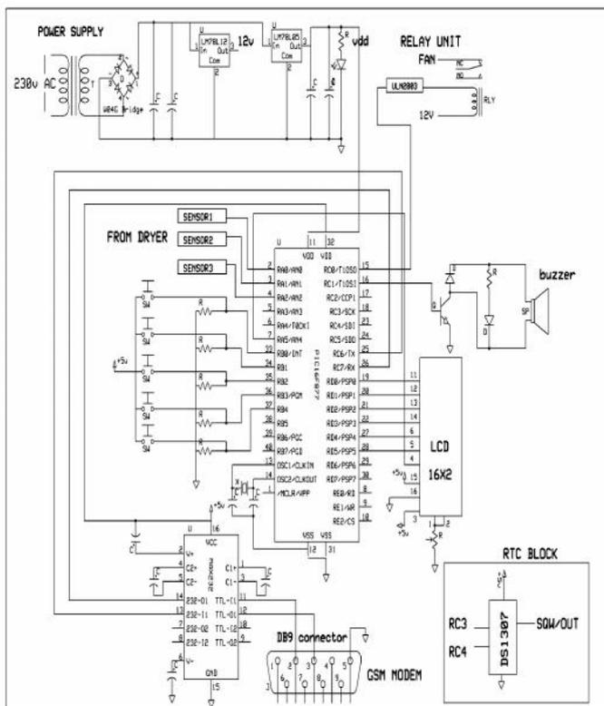
Fig.3. Drying controlling and monitoring circuit diagram
