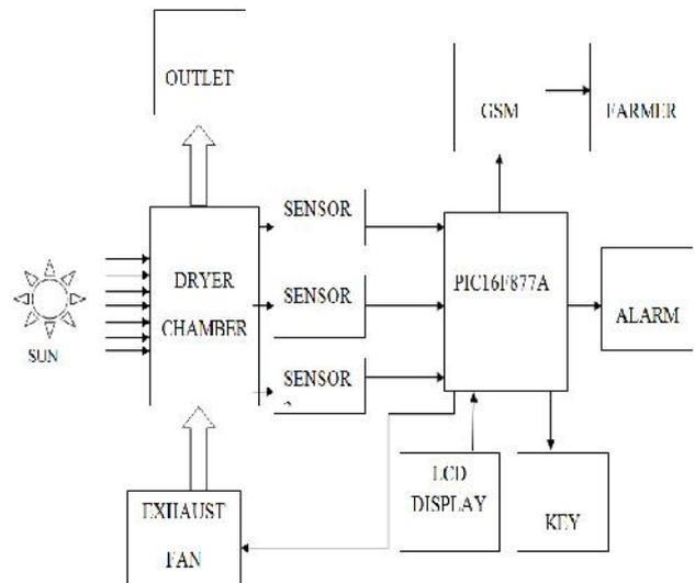
Fig.2. Automatic dryer system
