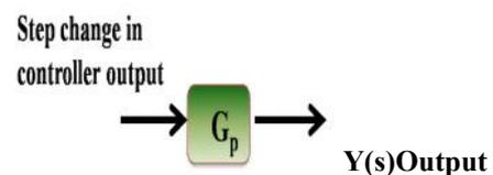
Figure 2: Block diagram of open loop response
