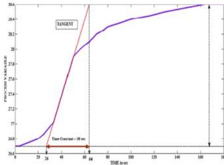
Figure 3: Response for a step change in controller output
