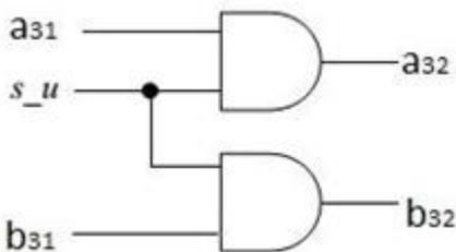
Fig.8. Logic Diagram of Sign Converter
