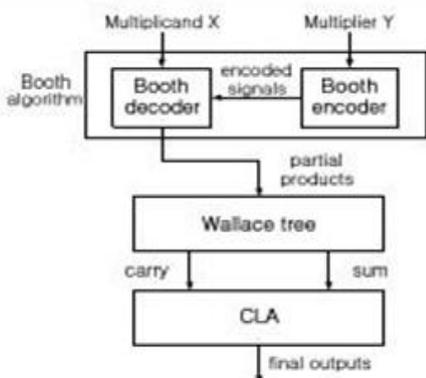
**Fig. 4** Architecture of the modified Booth multiplier.
