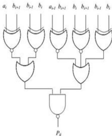
Fig. 6. Logic diagram of 1-bit partial product generator
