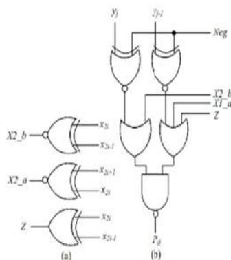
**Fig. 1. The Encoder and Decoder for the new MBE scheme. (a) Simple encoder (b) Decoder.**
