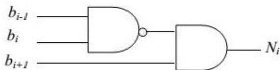
Fig. 7. Logic diagram of negate bit generator.
