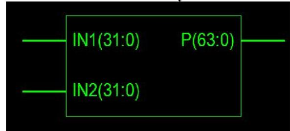
Figure 10: RTL Diagram Multiplier
