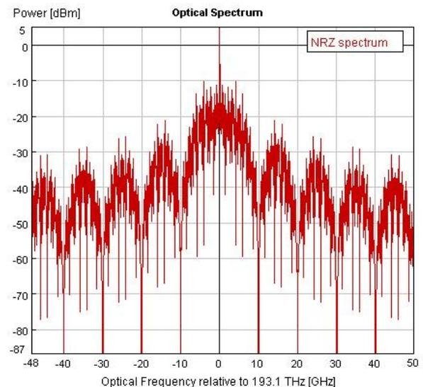
**Figure 1: Non return to zero (NRZ) modulation format**
