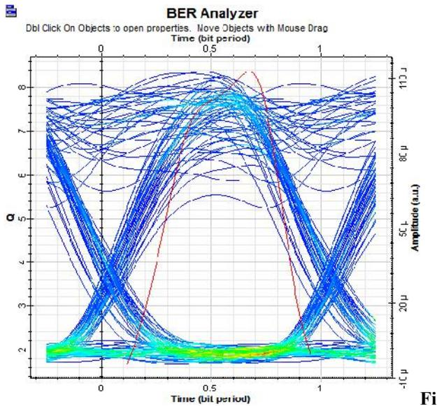
Figure 5: Eye Diagram of signal for dispersion compensation using Optigrating
