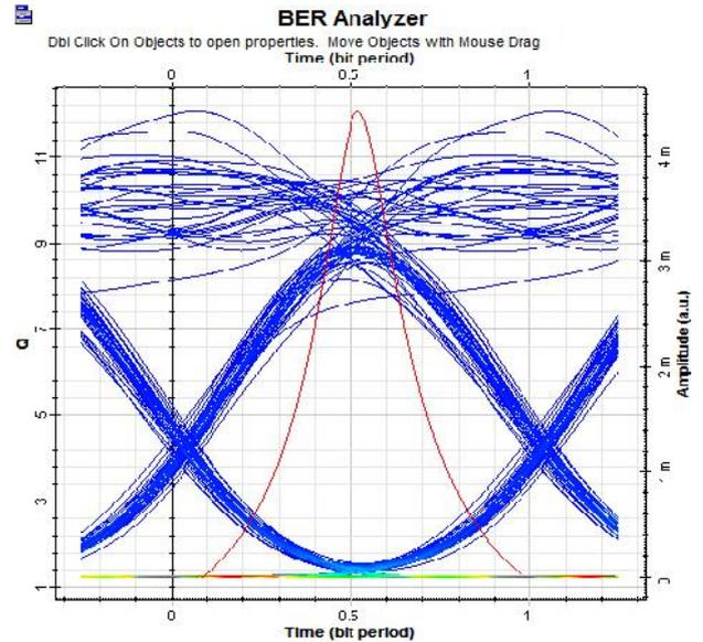
**Figure 4: EYE diagram of signal for dispersion compensation using Symmetrical DCF**
