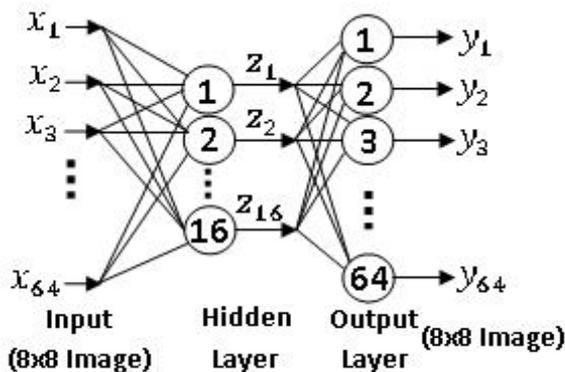
Fig 1. Architecture of feed forward neural network
