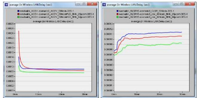
Fig 5: Avg. End-to-End Delay of AODV & OLSR without, with 25% & 50% attack for 50 nodes.
