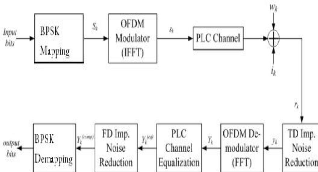
Fig 3.1 Block diagram of the OFDM-based PLC system with Joint TD/FD impulsive noise reduction
