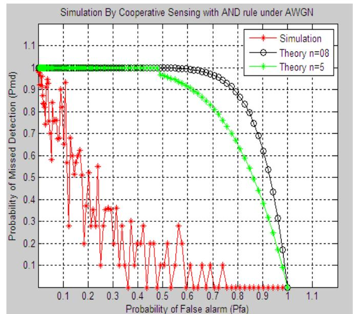
Fig: Simulated Test Results of Cooperative Sensing Method
