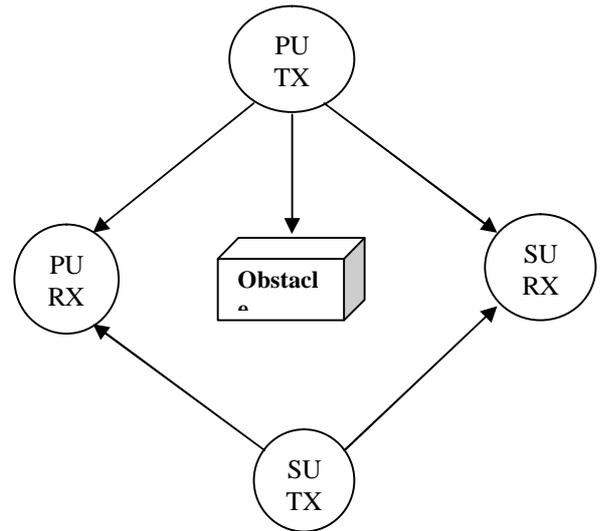
Fig 1: Hidden PU which cannot be detected by SU due to presence of obstacle.
