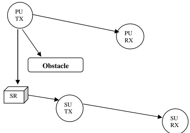
Fig 2: Use of SR, support SU to detect PU
