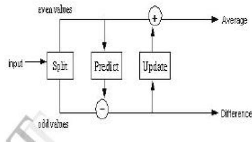
Fig 3: Lifting Scheme Process Flow It is composed of three basic operation stages:
