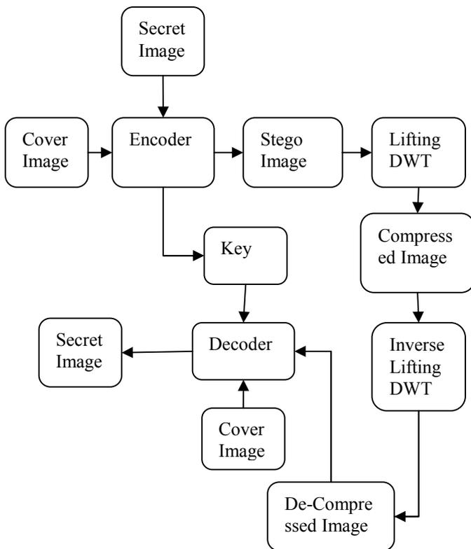
Fig 1: Overall Architecture Block Diagram Least significant bit (LSB) substitution
