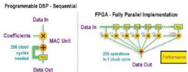
Fig 4: FPGA Vs DSP Processors Comparison
