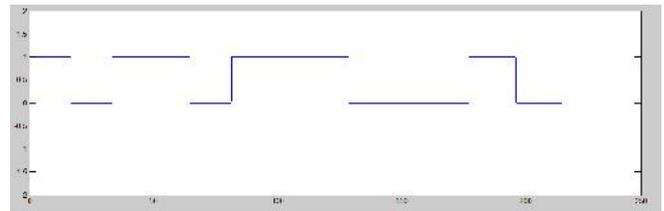
Fig.2: Input bit stream generated by Bernoulli random generator
