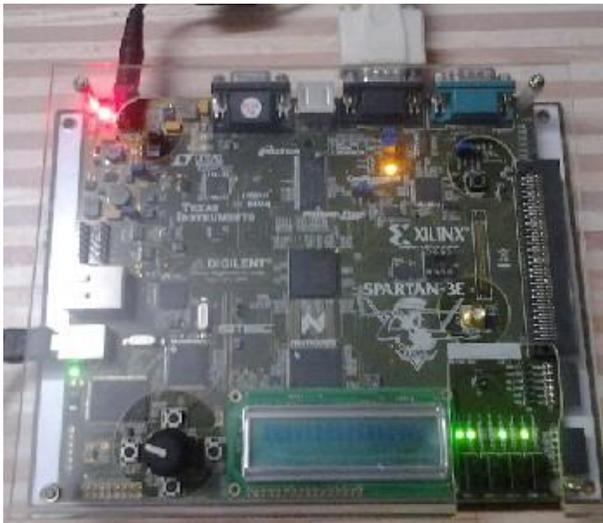
Figure 15. Xilinx Spartan 3E FPGA Board with Serial (RS-232) Communication
