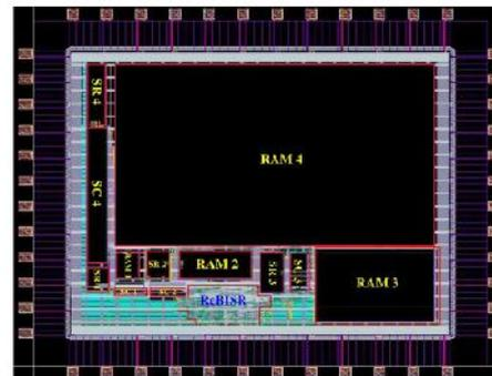
Fig. 15. Layout view of a ReBISR circuit for four RAMs.
