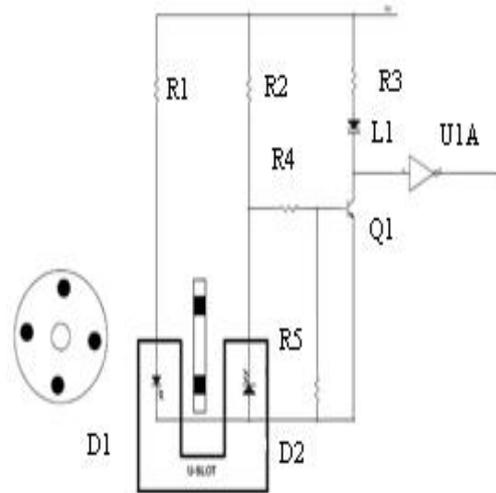
Fig.4 Speed measurement module
