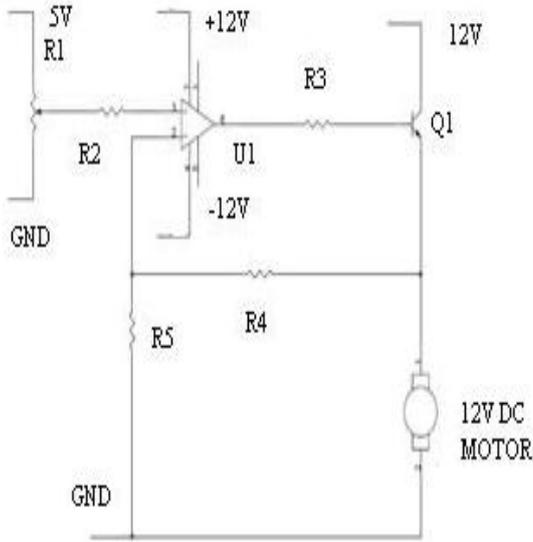
Fig.5 Speed Control module
