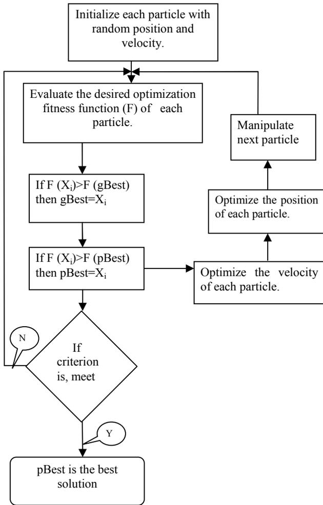
Fig 1: Flow diagram of PSO
