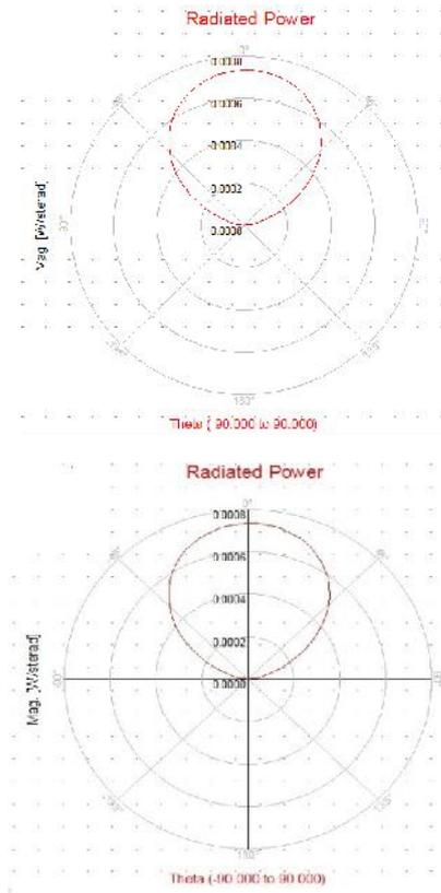
Fig.6Radiation pattern of proposed patch antenna at 6.07 GHz for xz-plane and yz-plane.
