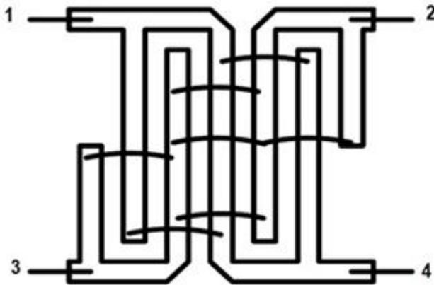
Fig.3 Microstrip Lange Coupler 6 fingered
