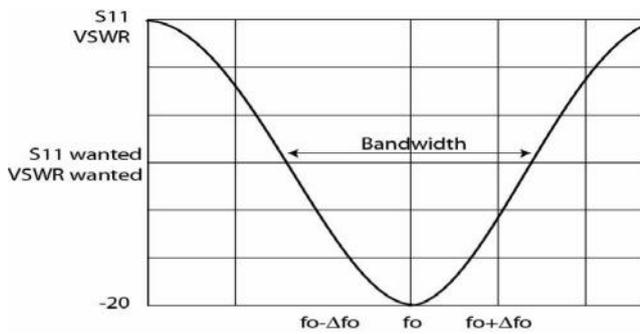
Fig.1 Return loss of patch antenna
