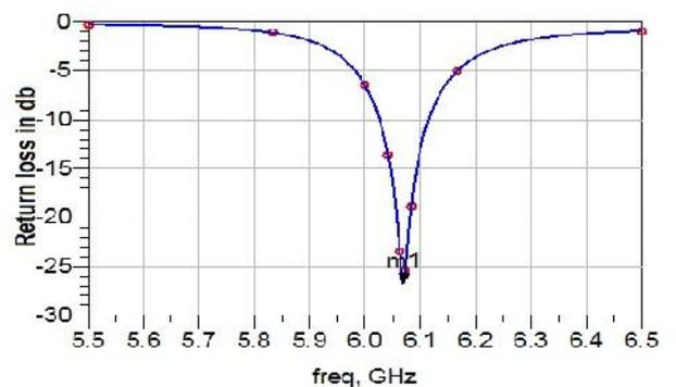
Fig.5 Simulated return loss of the proposed patch antenna.
