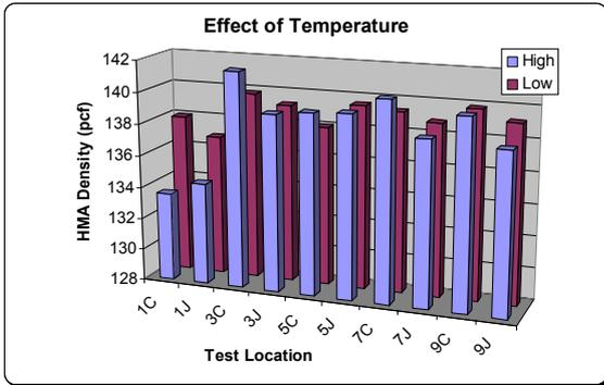
Figure 11. ASTM E 1169 Analysis – Effect of Temperature
