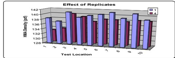
Figure 16. ASTM E 1169 Analysis – Effect of Number of Replicate Readings
