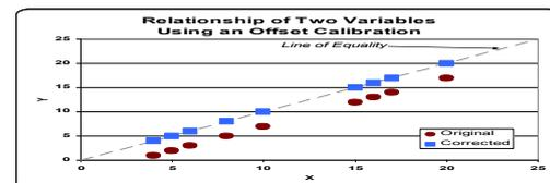
Figure 7. Relationship of Two Variables Using an Offset Calibration
