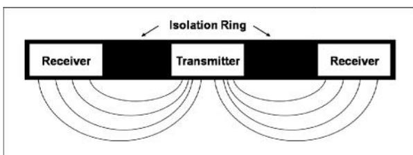
Figure 3. Schematic of Non-nuclear Gauge Function
