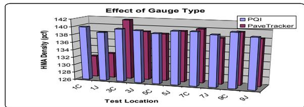
Figure 17. ASTM E 1169 Analysis – Effect of Number of Gauge Type
