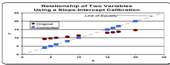
Figure 9. Relationship of Two Variables Using a Slope-Intercept Calibration
