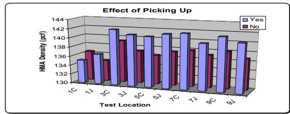
Figure 15. ASTM E 1169 Analysis – Effect of Picking Up the Gauge
