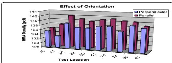
Figure 14. ASTM E 1169 Analysis – Effect of Gauge Orientation
