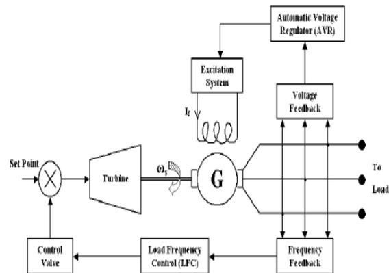
Fig. 02. Block diagram which is used for linear model with governor and AVR system.
