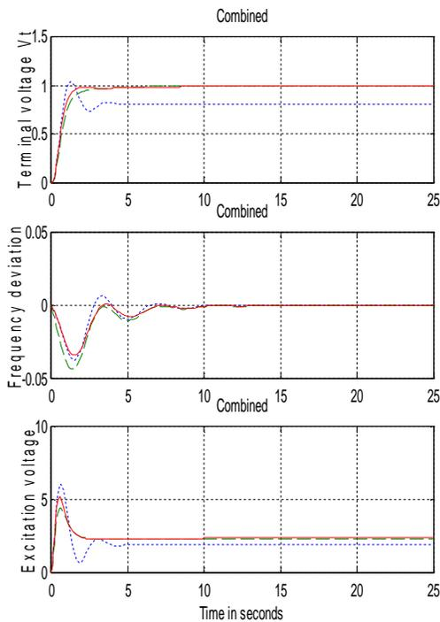
**Fig. 07: The collective/combined responses (Terminal voltages, Frequency deviations and Excitation voltages) with all controllers (Without controller, With PID, and With MLP) are shown.**
