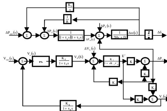
Fig. 03. Linearized model of governor and AVR excitation of synchronous generator with PID AVR excitation controller system
