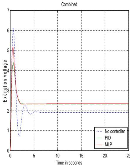
**Figure 06: Excitation voltages responses of: Without controller, PID, MLP controllers and collective excitation voltages responses (left, top to bottom) and in large response with collective controllers (right).**
