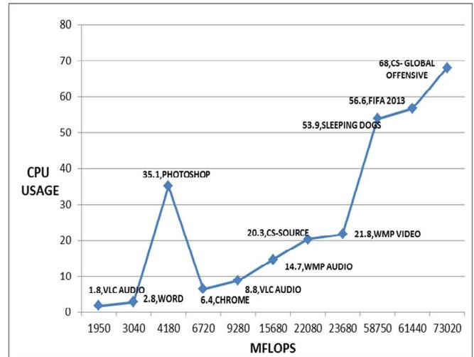
Fig 4 – Graph between CPU usages And MFLOPS (Million Floating Point Operations per Second) for various applications
