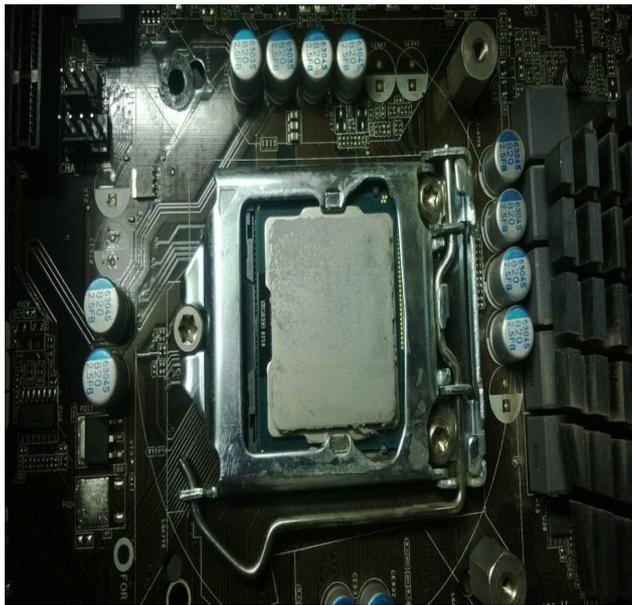
Fig.1 Intel I5 Microprocessor Installed in a Motherboard
