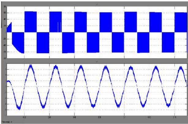
fig 12: MATLAB results showing inverter output voltage and output current
