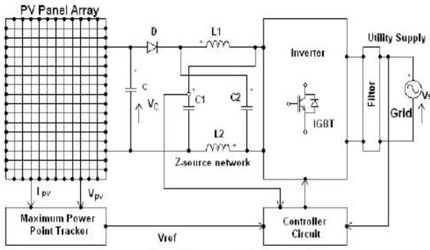
Fig. 2. Schematic diagram of a grid-connected PV system
