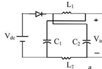
Fig .1 .Basic circuit of a z source inverter
