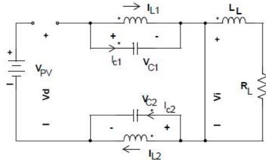
fig 3 Shoot-through zero state of a z-source inverter
