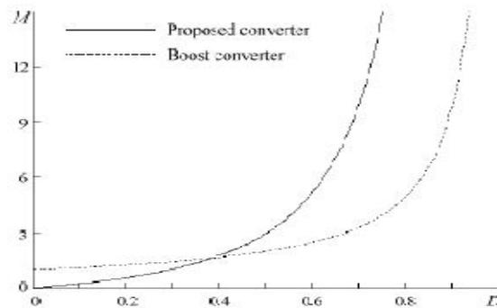
**Fig. 5. Voltage gains versus duty ratio for the proposed converter and the boost converter.**
