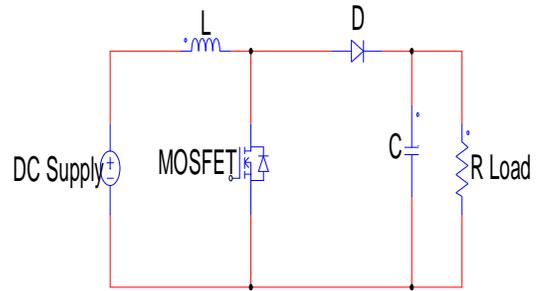
**Fig 7. Basic Circuit of Boost Converter**
