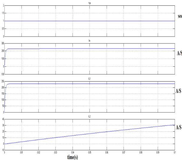
Fig 10. Waveforms of Closed loop Cascode Inductor Currents
