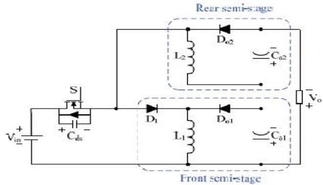
Fig. 2. Circuit configuration of the proposed converter.
