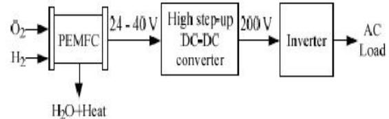
Fig. 1. Fuel-cell electric conversion system.
