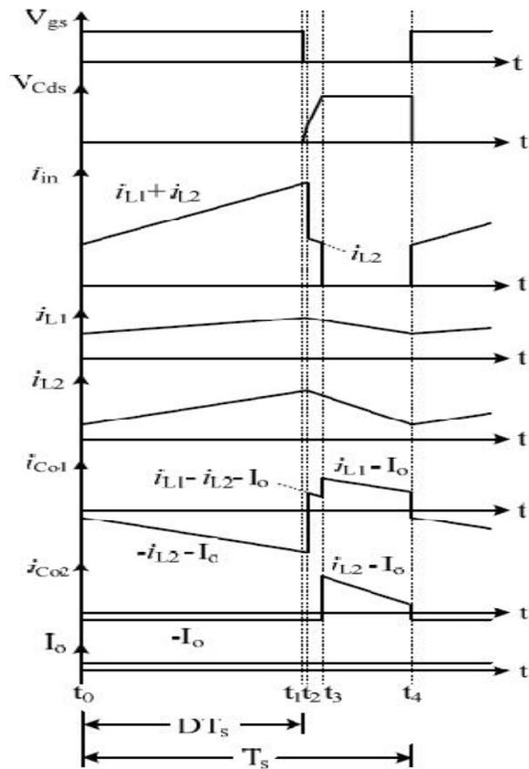
Fig. 3. Typical waveforms of the proposed converter in CCM operation.
