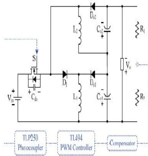
**Fig. 6. Prototype circuit of the proposed cascode converter.**
