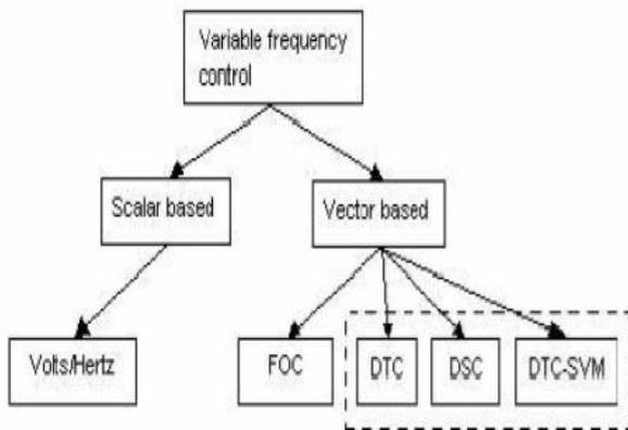
Figure 2.1, Some common control techniques used for PMSM. Control methods in the dashed box belong to the DTC family
