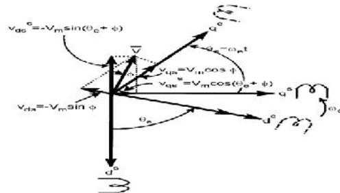
Fig 3.1(b) stationary frame d<sup>s</sup>-q<sup>s</sup> to dynchronously rotating frame d<sup>e</sup>-q<sup>e</sup> transformation
