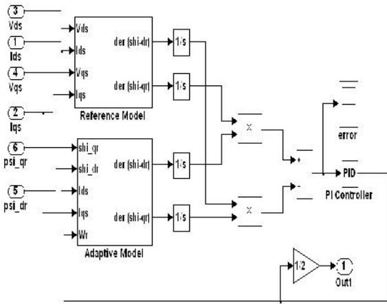
Fig 12: Simulink block diagram for Model Referencing Adaptive System with pi
