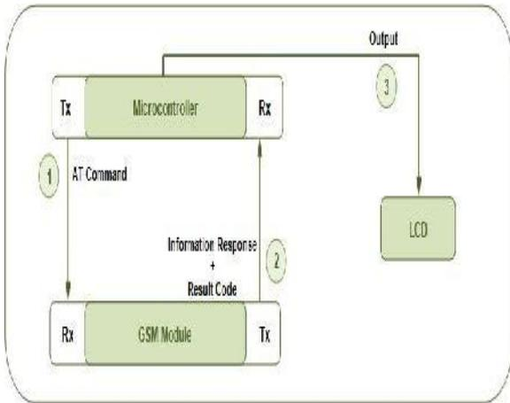
Fig.5 Interface between modem and microcontroller
