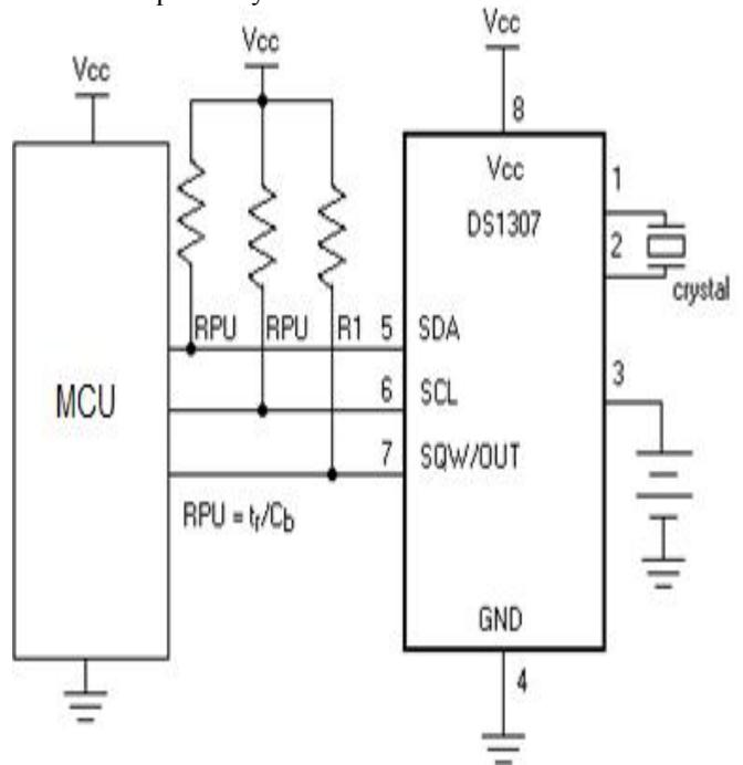
Fig.4 Connection Diagram of Real Time Clock
