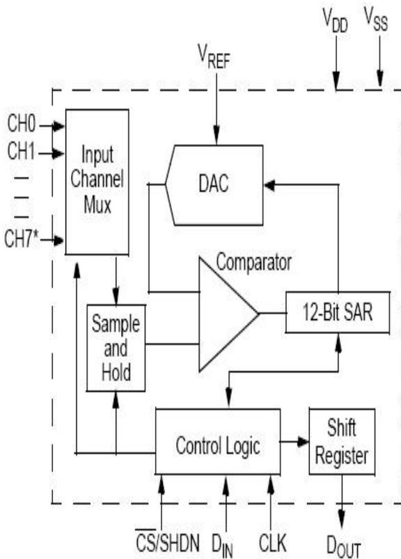
Fig.3 Functional Block Diagram of MCP3208 ADC
