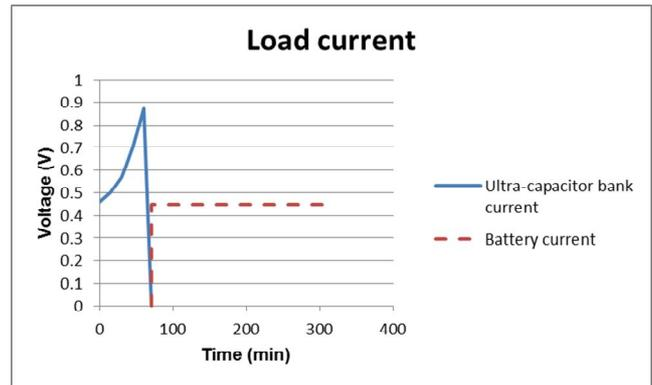
Fig. 11. Battery and super-capacitor load current.
