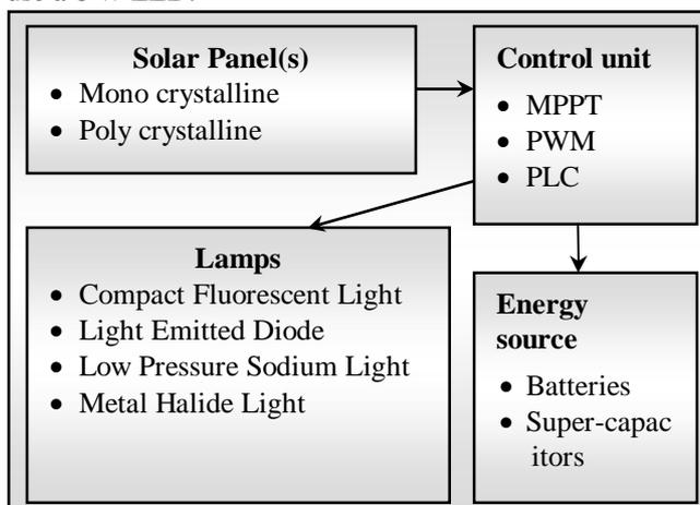
Fig. 1. Conceptual design of the PV streetlight.
