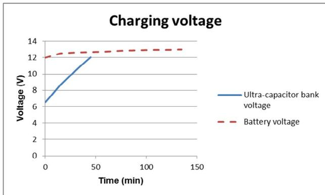
Fig. 9. Battery and super-capacitor charging profiles.
