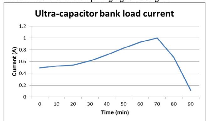
Fig. 7. Super-capacitor load current profile.
