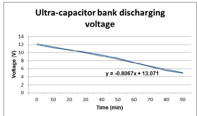
Fig. 6. Super-capacitor discharging voltage profile.
