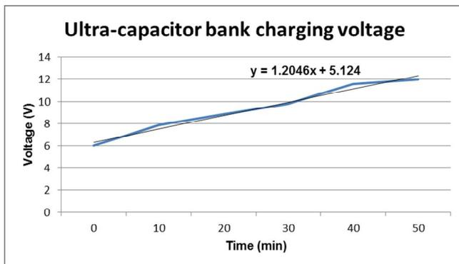
Fig. 5. Super-capacitor charging voltage profile.
