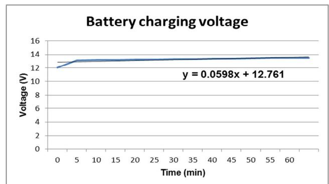
Fig. 3. Battery charging voltage profile.
