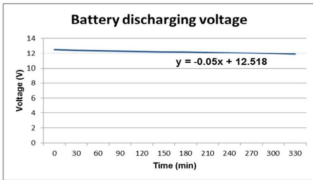
Fig. 4. Battery discharging voltage profile.
