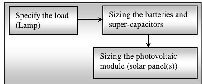
Fig. 2. Design methodology of the PV streetlight.
