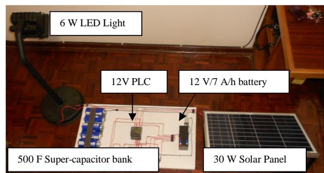
Fig. 8. Experimental test setup system.
