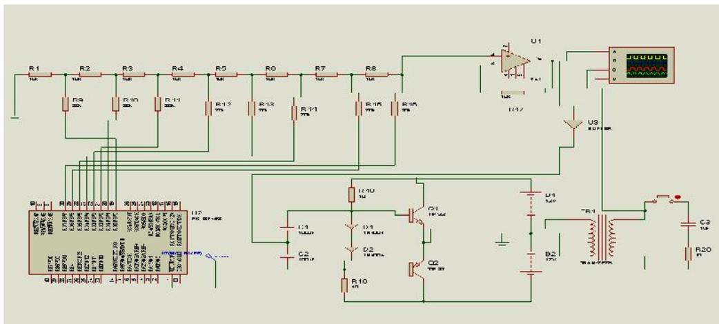
**Fig 2 Variable frequency high voltage sine wave generation**
