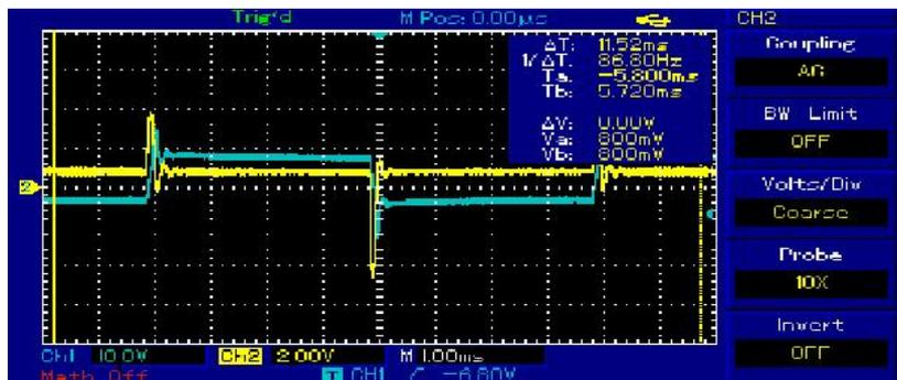
Fig 5 Typical waveform of the leakage current variation during a breakdown
