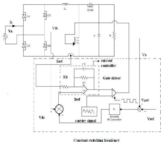
Fig. 1 Circuit Configuration of PFC Converter with ACMC.
