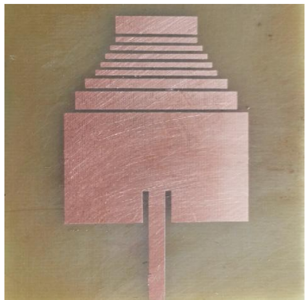
Fig.7 Fabricated Yagi Uda shaped frequency Reconfigurable microstrip antenna
