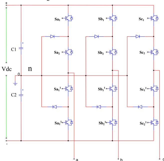
**Fig 2. Three-phase three level diode clamped inverter**
