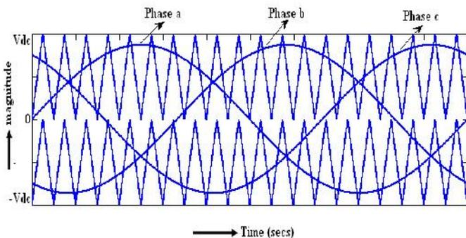
**Fig 7. SPWM with triangular multilevel carriers**
