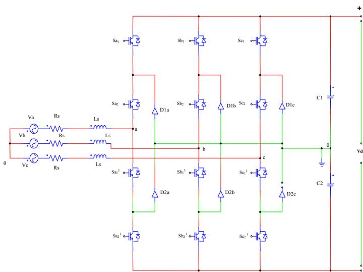
Fig 4. Three-phase three level diode clamped Rectifier
