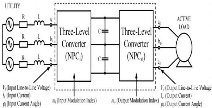
**Fig 6. Back-to-back application of NPC converters.**
