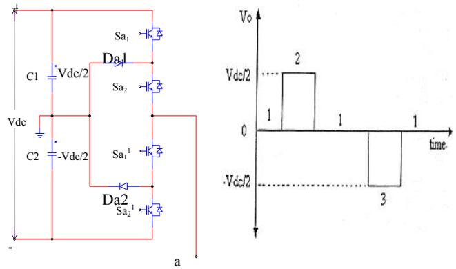
**Fig 3(a). One phase of three level diode clamped inverter**
