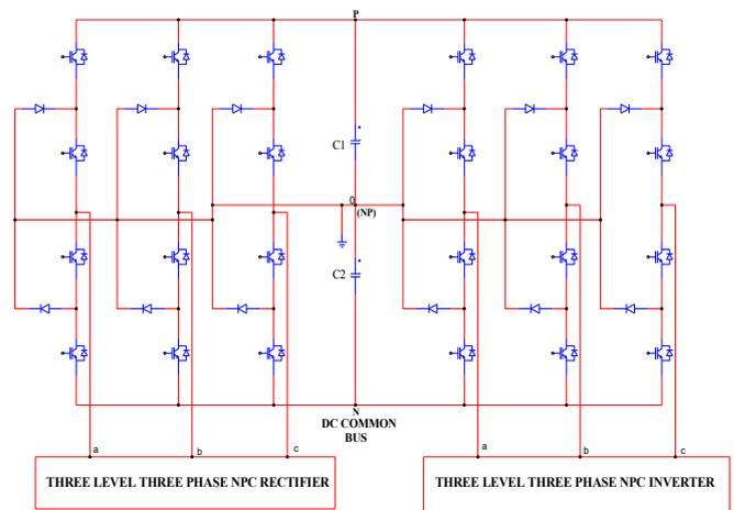
**Fig1. Three-level three-phase back-to-back converter.**
