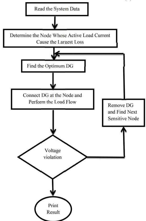
Step 3: A load flow is performed in order to get the new values of the load currents and to check if the voltage constraints are met. If there is any violation of the voltage constraints, the DG is removed and the next largest loss node is selected as the next sensitive node and the procedure is repeated starting from Step 2.
