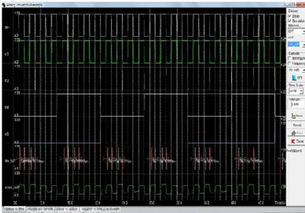
Figure 8 Waveform for CMS-bias with d-latch as a delay element
