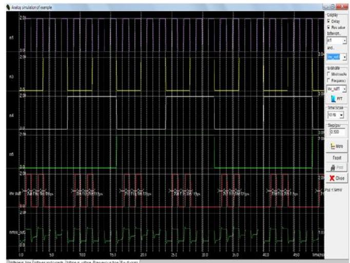
Figure 7 Waveform for CMS-bias with Buffer as a delay element
